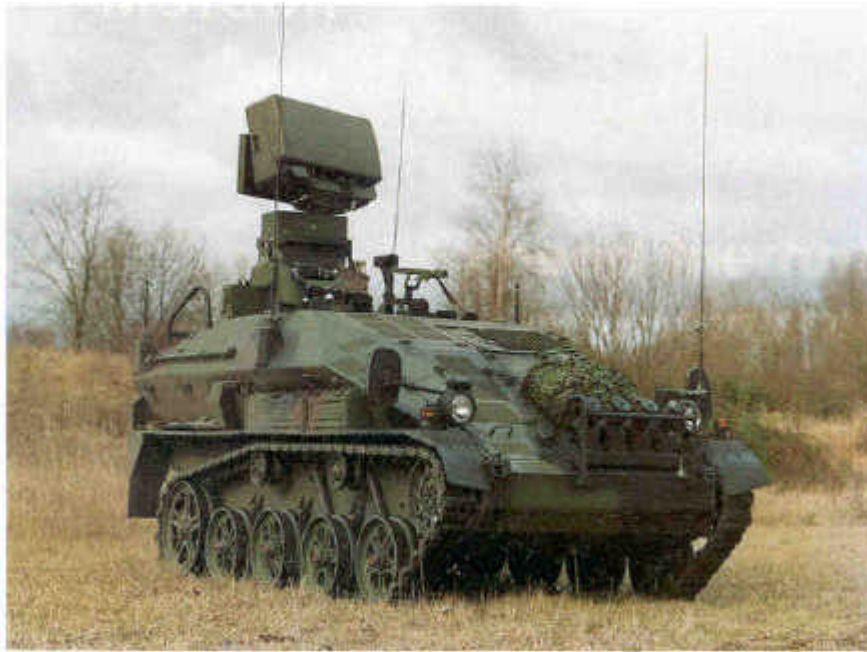
HARD Radar Mounted on German MaK Wiesel 2 Surveillance Vehicle
